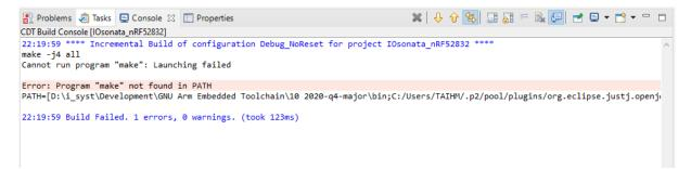
If you are using GNU MCU Eclipse on Windows, make sure <u>Windows Build Tools</u> are installed, then check the installation path and fill the "Global Build Tools Path" inside Eclipse Window/Preferences... :
